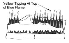
Figure 37 - Incorrect Front Burner Flame Pattern
